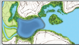
Potential location of upstream sediment forebay
